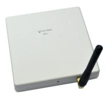
The control panel is part of the heat management system, designed to control the C.O boiler. (eg gas, oil, coal), which is equipped with a thermostat input. The control panel controls 230VAC thermoelectric actuators based on the radio temperature sensors in the VRC thermostatic heads. The control panel supports up to 12 heating zones.
