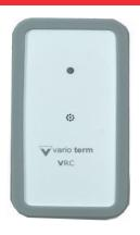
Wireless temperature and humidity sensor is a device that allows you to precisely control the temperature in a specific zone of the room. In addition, the sensor measures the humidity, which gives us the knowledge if the heating is not too dry. The sensor sends information about measurements to the controller via radio to the VRC system.
